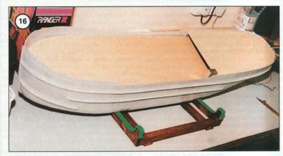
hatch. I was then able to mark out and cut out the main hatch.
