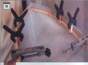
a correct line, make up a small gauge from plywood and insert a pencil at the correct depth and then run the gauge around the inside of the hull as in Photos 6 and 7. Start by fitting the strip-wood around the sweeping parts of the hull and when the bow and stern parts are reached, slots can be cut into the strip-wood so that the shapes can be easily fitted as shown in Photos 8, 9 and 10. When the glue has set on
